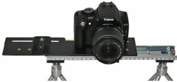
Fig. 4 Triaxes StereoRail tripod for stereo multiview photo and video shooting (source - www.triaxes.ru )
