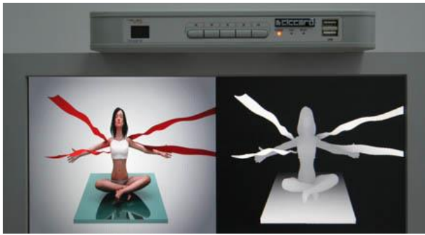
Fig. 7 Elecard 3DSTB prototype. MPEG-2 1080 HD video stream decoding in the 2D+Z format.
