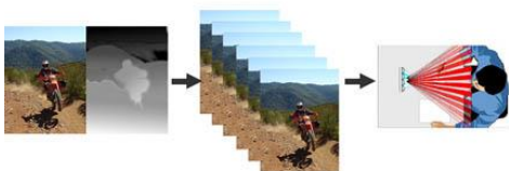
Fig. 6. 2D+Z image transformation into a frame series and its demonstration on a 3D display (source - www.philips.com , www.isu3d.org ).
