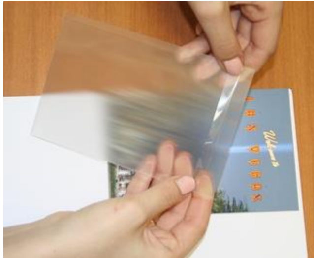
Fig. 4.16 Fold up 1 cm of the protective film
