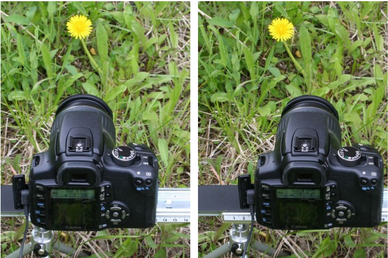
Fig. 2. Multi-frame shooting with one camera (the leftmost and the rightmost positions are shown)
